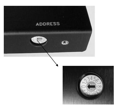
Figure 5. Address Selection Switch
