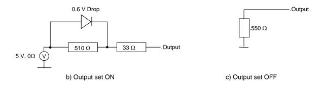
Figure 2. Simplified Equivalent Port Circuits and Graphs of Output Voltage
